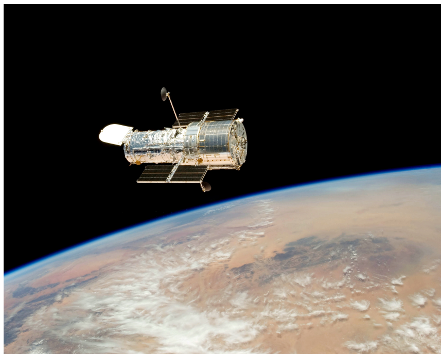
5. Hubble Space Telescope orbiting Earth at 593 km above sea level.
